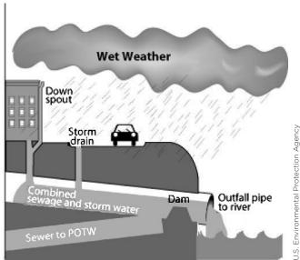
During rain storms, runoff can overwhelm the capacity of combined sewers, sending untreated sewage and runoff into local waters.
