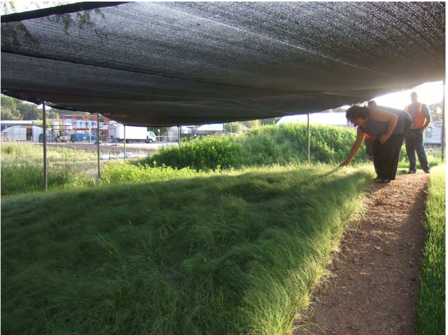
A shaded lot in a 8,150-square-foot mock-up of the native lawns at the George W. Bush Presidential Center, a study led by Laura to test slope retention, planting soils, shading, and irrigation
