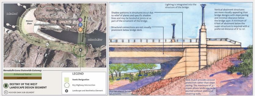
Scenic designation design objectives were an essential recommendation for US 93 ^ Bridge abutments and barrier rails are designed as a composition with jointing and materials consistently applied. crossing the Hoover Dam and the Colorado River.
