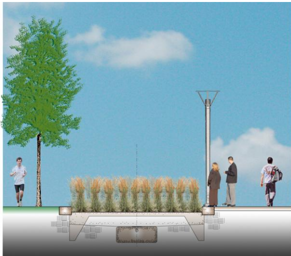
Figures 2 & 3- Cross section of bioswale and as installed.
